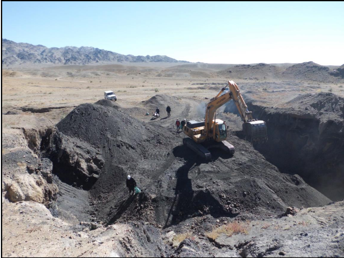
Collecting bulk sample from historical open pit, KZ Metallurgical Coal Project
